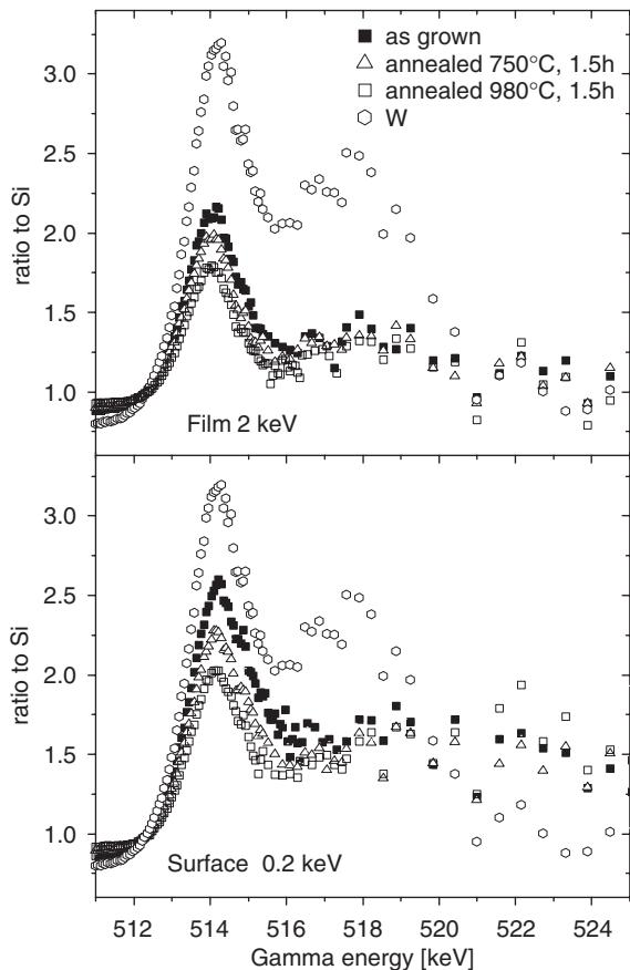
Fig. 2. Coincidence ratio curves referred to Si. The curves were measured in the samples of the series  $\text{W}_{40}\text{Si}_{18}\text{N}_{42}$  at 0.2 and 2 keV corresponding to a depth of 0.4 and 15 nm, respectively. The W ratio curve to Si is also shown.
