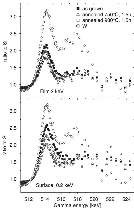
Fig. 2. Coincidence ratio curves referred to Si. The curves were measured in the samples of the series  $W_{40}Si_{18}N_{42}$  at 0.2 and 2 keV corresponding to a depth of 0.4 and 15 nm, respectively. The W ratio curve to Si is also shown.
