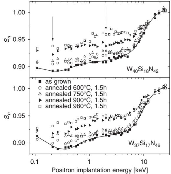
Fig. 1.  $S_n$  vs. positron implantation energy for  $W_{40}Si_{18}N_{42}$  and  $W_{37}Si_{17}N_{46}$  films as-grown and thermal treated. The arrows mark the energies where C-DBS curves were measured. As an example the best fits for the as deposited samples of both series are reported.
