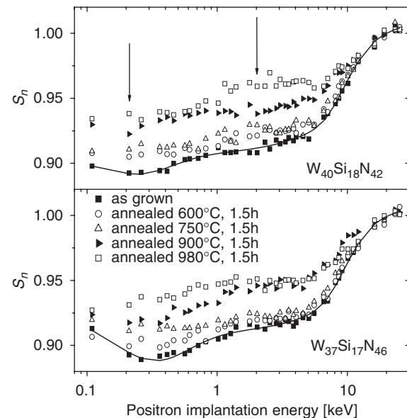
Fig. 1.  $S_n$  vs. positron implantation energy for  $\text{W}_{40}\text{Si}_{18}\text{N}_{42}$  and  $\text{W}_{37}\text{Si}_{17}\text{N}_{46}$  films as-grown and thermal treated. The arrows mark the energies where C-DBS curves were measured. As an example the best fits for the as deposited samples of both series are reported.
