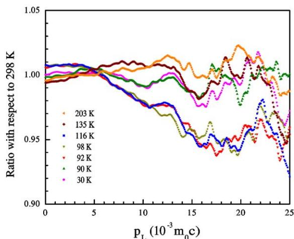
Fig. 1. Ratios of the experimental electron–positron momentum distributions at different sample temperatures to the electron–positron momentum distributions at the room temperature (298 K) for the single crystalline Bi-2212 HTSC.
