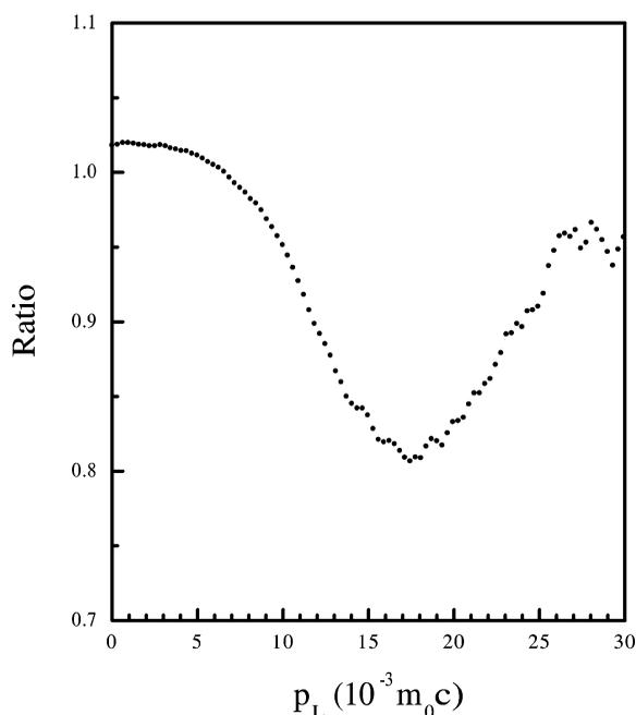
Fig. 2. Ratio of the experimental electron–positron momentum distributions for the nano-crystalline CuO powder to the electron–positron momentum distributions for the micro-crystalline CuO powder.
