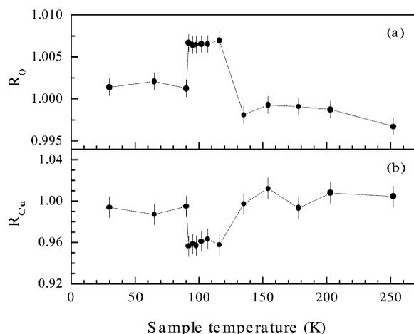
Fig. 3. Variation of the area-parameters (a)  $R_O$  and (b)  $R_{Cu}$  with sample temperatures for the single crystalline Bi-2212 HTSC.
