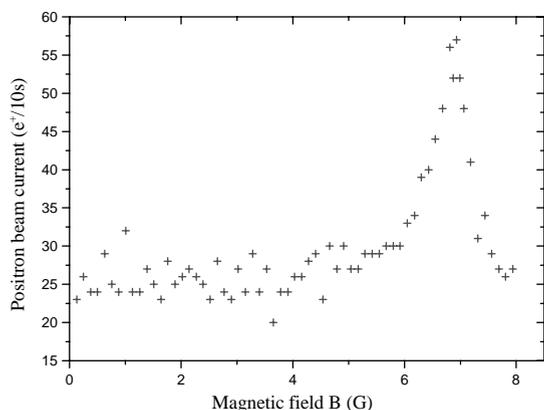
Fig. 3. Apparatus transmission function as measured with a positron beam: note the scale change. The position of the peak is different from the position in Fig. 2 due to the different emission energies.
