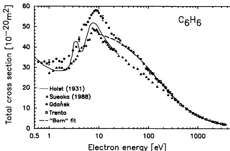
Fig. 1. Total cross sections for electron scattering on benzene molecule. (●) Present measurements (Gdańsk); (□) present measurements (Trento); (Δ) Sueoka [19]. Solid line: Holst and Holtmark [2]; dashed line: present intermediate-energy fit, Eq. (3). Error bars in selected points correspond to the total (systematic + statistical) experimental uncertainty. Error bars above 200 eV are smaller than the symbols.
