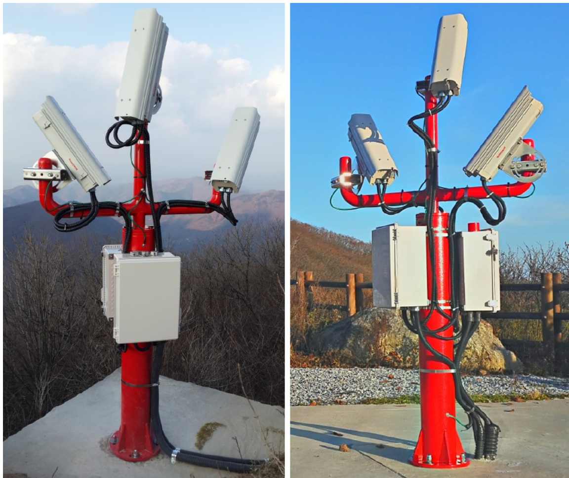
Fig. 6A: Double-station sky-monitoring camera system for the optical detection of meteors and fireballs in South Korea (left panel: BOAO site; right panel: SOAO site). The figure is reproduced from Hinse et al. (2017, Fig. 2).
