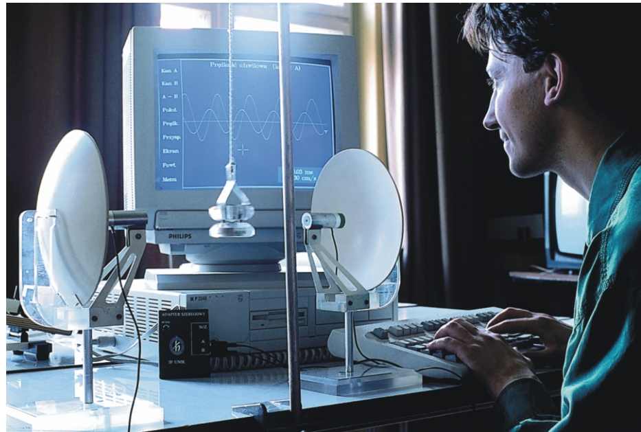
Ultrasonic motion detector constructed in EPL
