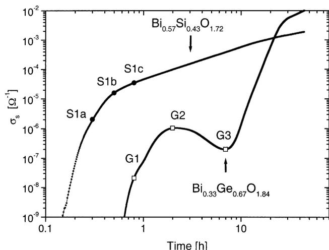
Fig. 1. Changes in the surface conductivity for silica-based (“S” series) and germanium-based (“G” series) bismuth-doped glasses (adapted from Ref. [2]) during heat treatment at 340 °C.
