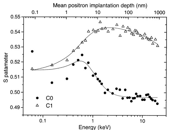
Fig. 7. The  $S$ -parameter for lead-silicon glasses (series V). Modelling of the  $S$ -parameter performed using the VEPFIT [11] program.
