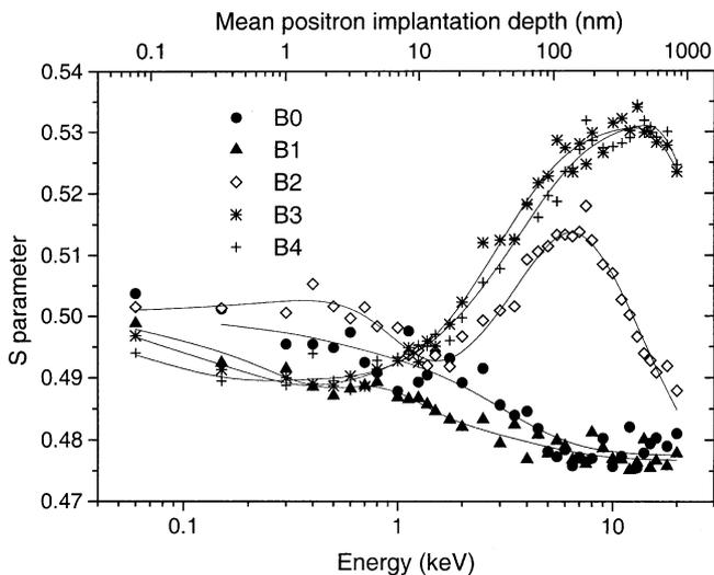
Fig. 5. The  $S$ -parameter for bismuth-germanium glasses (series III). Note a complex change of the  $S$ -level with the reduction time for the first 10 nm depth.
