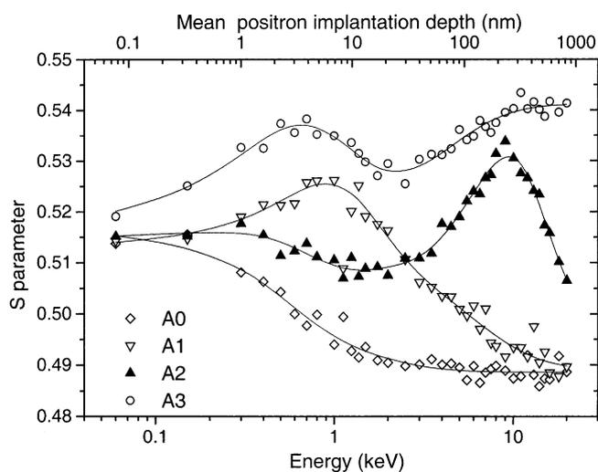
Fig. 3. Positron-annihilation  $S$ -parameter vs. positron implantation energy for bismuth-silica glasses (series I, with Si molar contents higher than Bi). Modelling of the  $S$ -parameter curves, has been performed using the VEPFIT [11] program. Increase of  $S$ -parameter in the formed reduced layer with rising reduction time is clearly seen.
