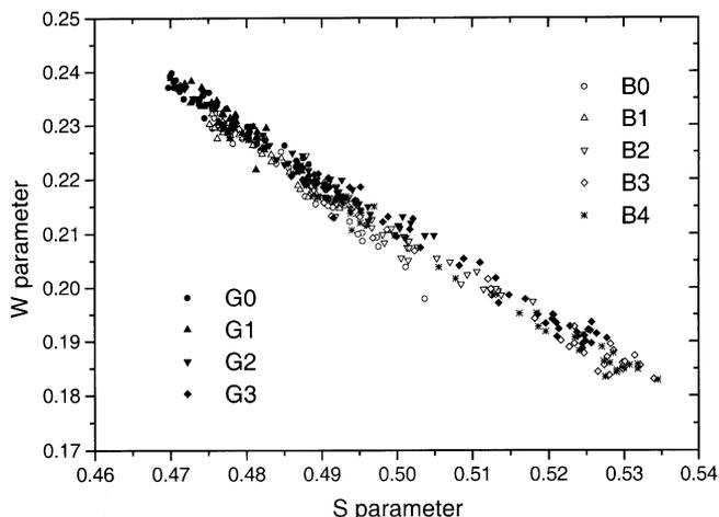
Fig. 9. Positron annihilation  $W$  vs.  $S$  plot for selected bismuth-germanium glasses (series III and IV). These data show a bigger scatter than the data from Fig. 8, but all of them lay in the same region of the  $S/W$  plane, indicating a similar nature of trapping centres in both samples.
