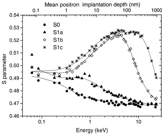
Fig. 4. Positron-annihilation  $S$ -parameter vs. positron implantation energy for bismuth-silica glasses (series II, with majority of Bi). Modelling of the  $S$ -parameter curves has been performed using the VEPFIT [11] program.
