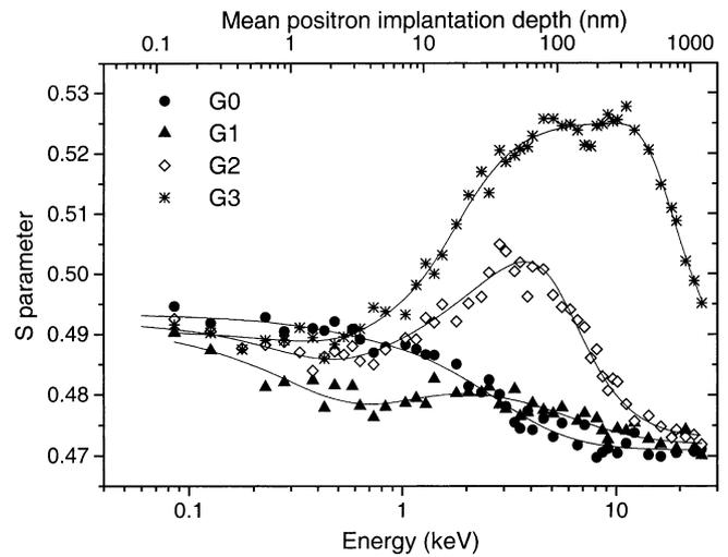
Fig. 6. The  $S$ -parameter for bismuth-germanium glasses (series IV, similar to series III).
