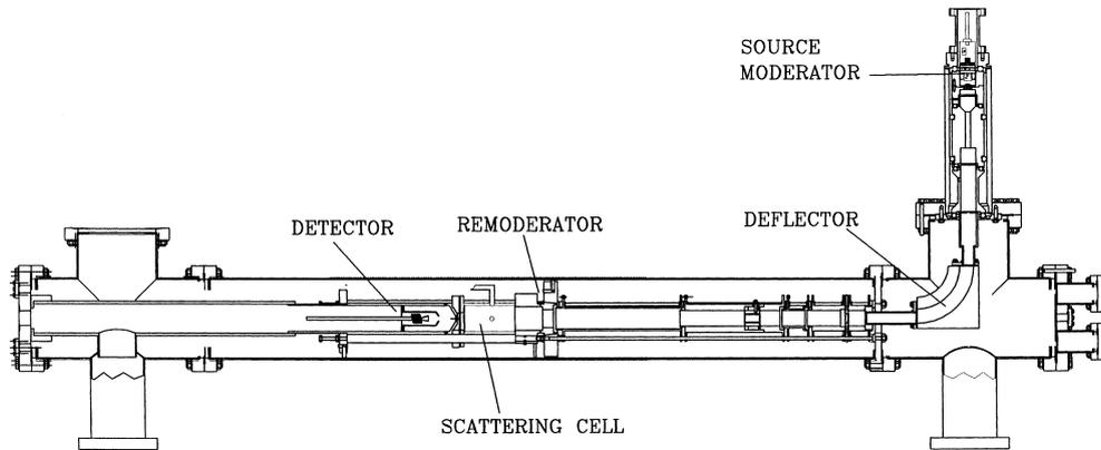
Fig. 1. Schematic drawing of the low-energy positron spectrometer.
