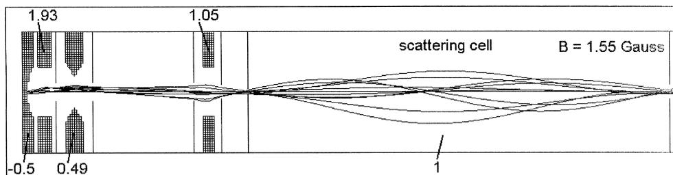
Fig. 2. Ray-tracing for a positron scattering energy of 1 eV. The voltages of the electrodes are given in  $V$ . The guiding magnetic field is  $1.55 \times 10^{-4}$  T. Hatched regions show the electrodes, real apertures are shown by vertical thin lines.
