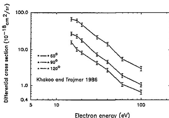
**Figure 2.** Elastic differential cross sections for electron scattering on  $\text{H}_2$  (from Khakoo and Trajmar 1986). Absolute values were obtained by normalization to  $e^- + \text{He}$  and  $e^+ + \text{Ne}$  values simultaneously. The error bars correspond to relative experimental uncertainties.
