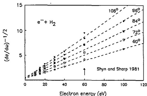
Figure 3. Plot of  $(d\sigma/d\omega)^{-1/2}$  in  $(10^{-20} \text{ m}^2 \text{ sr}^{-1})^{-1/2}$  units against energy. Data from Shyn and Sharp (1981). First-order regression lines are drawn through the 10–40 eV and 100 eV points. Notice that the 60 eV points depart from the regression values lines towards lower values of the cross sections.
