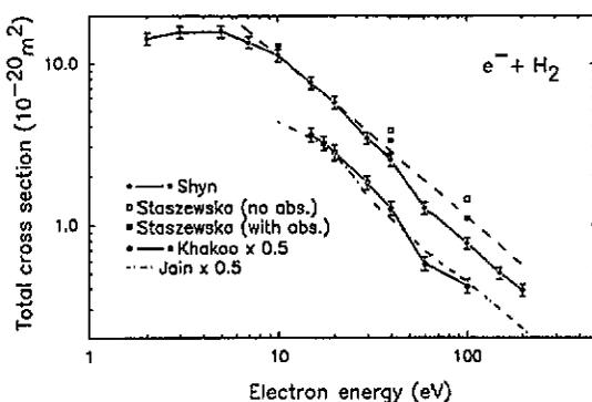
**Figure 4.** Integrated elastic cross sections for  $e^- + \text{H}_2$  scattering: full circles, Shyn and Sharp (1981); open circles, Khakoo and Trajmar (1986); the error bars correspond to integration errors; chain curve, optical potential calculations of Jain and Baluja (1992); full squares, optical model without absorption (Staszewska *et al* 1984); open squares, the same model with absorption. The broken curve indicates the  $1/E$  dependence drawn through the 20 eV point.
