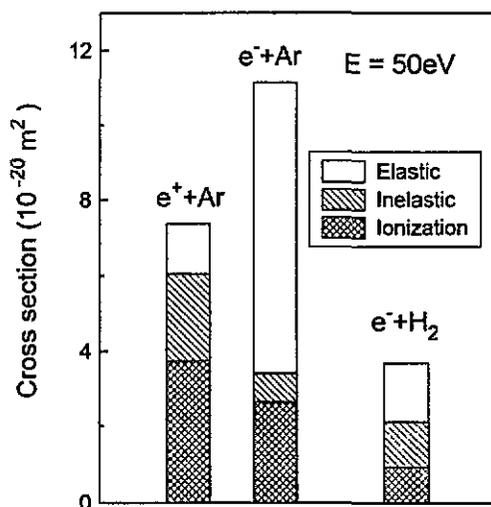
**Figure 1.** Partitioning scheme for electron and positron scattering on argon and hydrogen at 50 eV:  $e^+ + \text{Ar}$ , ionization from Knudsen *et al* (1990) corresponding to ionization + electronic excitation of Mori and Sueoka (1994); inelastic = positronium formation from Fornari *et al* (1983) corresponding to the 'lower limit' for positronium formation of Zhou *et al* (1994); elastic is that obtained by subtraction of the two above values from the total one (Stein *et al* 1992).
