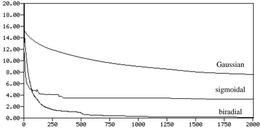
Figure 6: Comparison of the summed squared errors for different transfer functions: Gaussian (Eq. 14), sigmoidal (Eq. 2) and biradial function (Eq. 35) used in the same RBF net during 2000 epochs.
