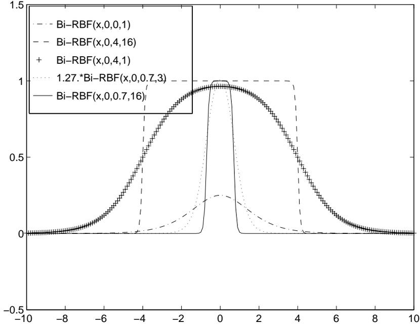
Figure 4: A few shapes of the biradial functions in one dimension.
