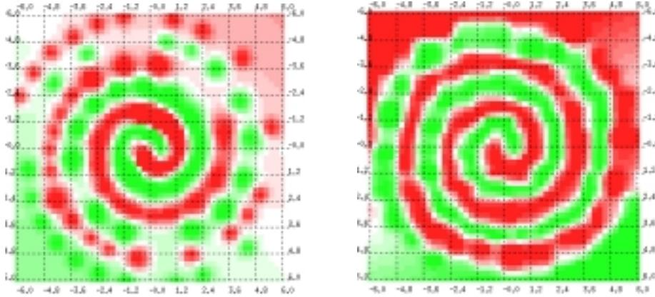
Figure 5: Results for the two spiral classification problem solved with the Gaussian (left figure) and biradial (right figure) transfer functions.
