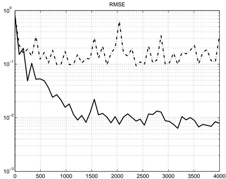
Figure 7: Comparison of RMS errors obtained by the IncNet network using biradial (solid line) and Gaussian (dashdot line) functions.
