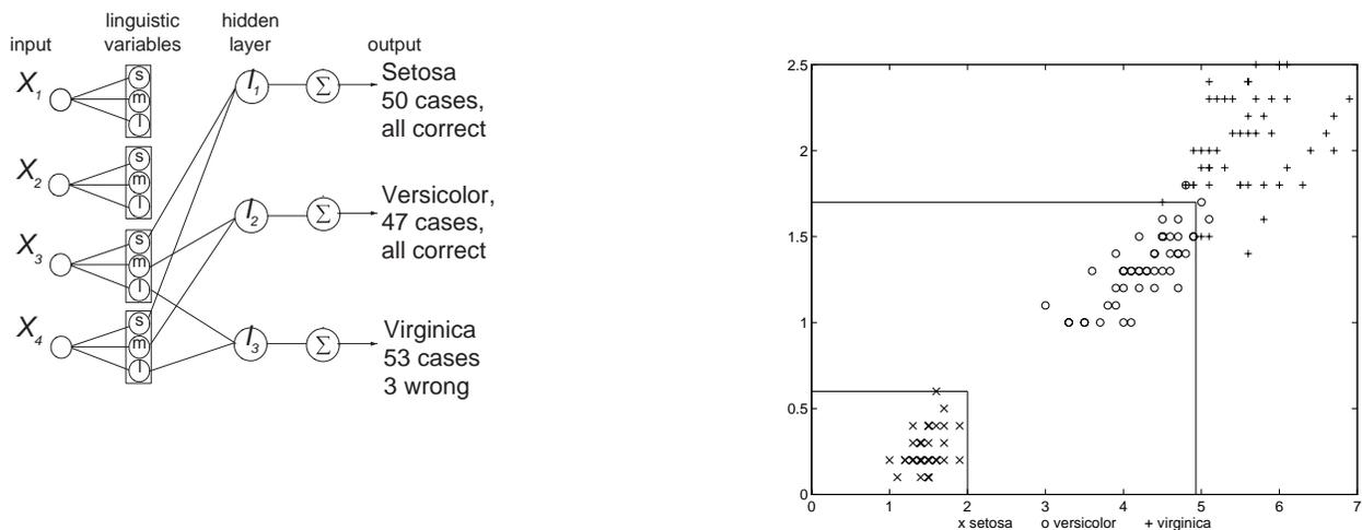
Fig. 2. Final structure of the network for the Iris problem and the decision borders in the space of the two relevant features  $x_3$  and  $x_4$ .
