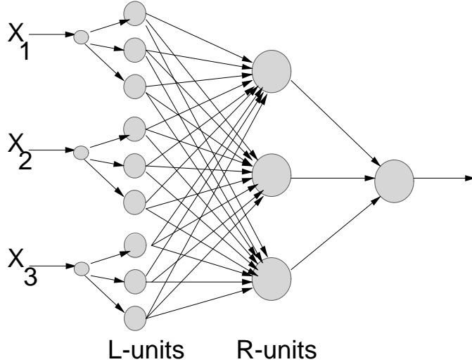
Fig. 2. Structure of the network for rule extraction and feature selection. *L*-units convert continuous inputs into linguistic variables, *R*-units form the rules.
