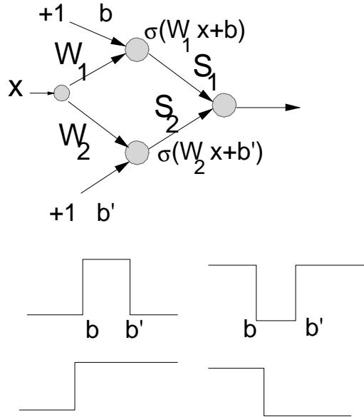
Fig. 1. Construction of a linguistic unit converting continuous inputs to linguistic variables.
