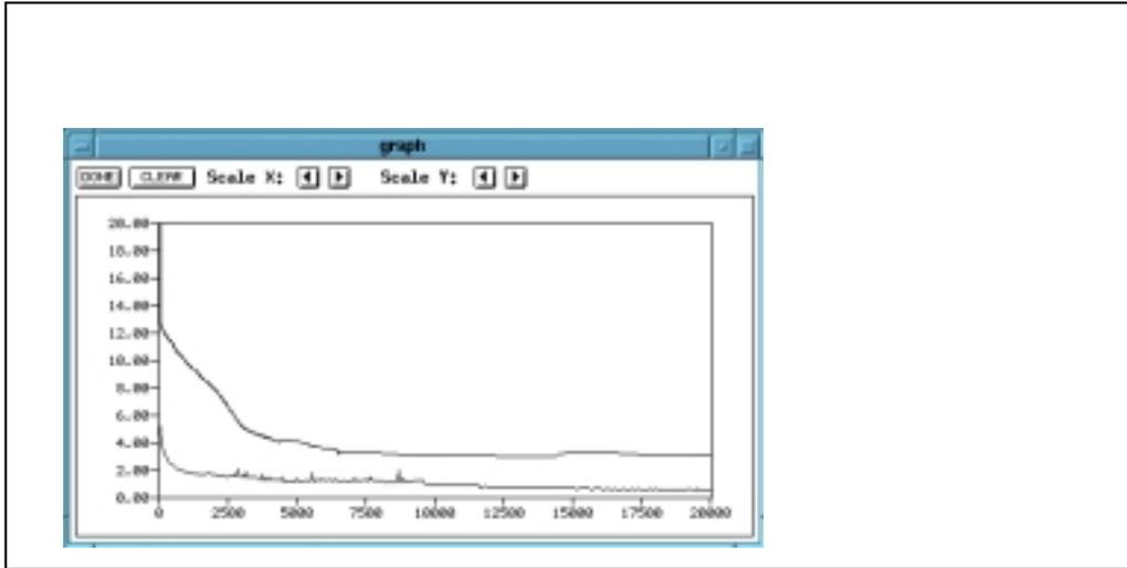
FIG. 3. Convergence rate of the RBF (upper curve) and FSM (lower curve) on the two-spiral benchmark with 100 nodes.
