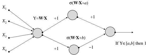
Figure 1: Basic processing element replacing several neurons that share weights and have inhibitory connections.
