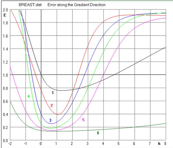
**Fig. 3.**  $\Delta w < \text{optimal } \Delta w$  in continuous or mixed NG; errors along the gradient direction for 6 training cycles. Horizontal axis (h): distance in the gradient direction from the starting point ( $h=0$ ) for each training cycle. Vertical axis (E): relative MSE ( $\text{MSE}=1$  when the training starts) (breast cancer data)
