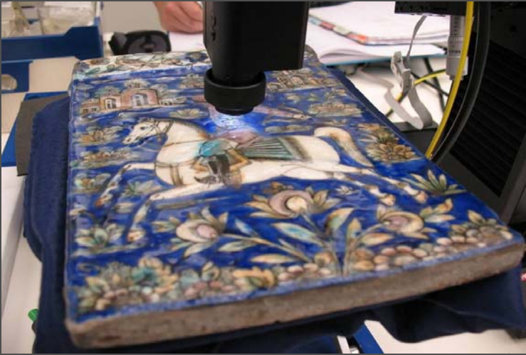
Non-invasive examination of BM G.313 by OCT using equipment from Nottingham Trent University
